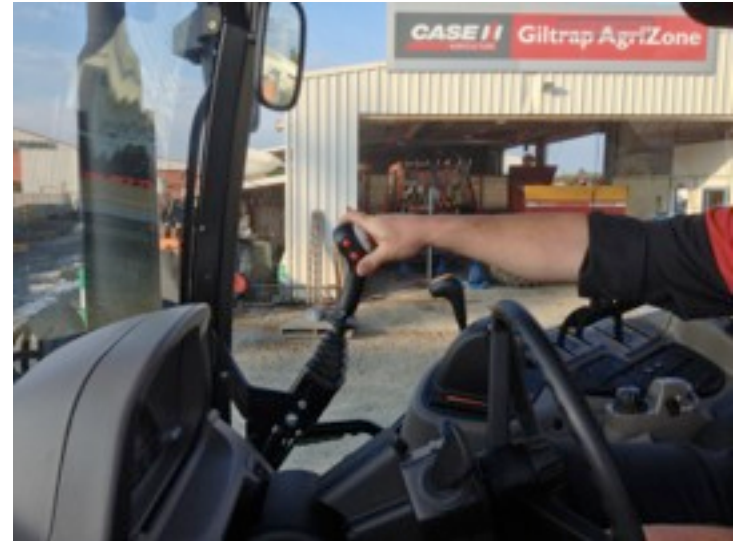
12). Release the Hand Brake. Crowd the Joystick Forward until the Loader Drops into place and the Safety Lock Pins click into Position.
