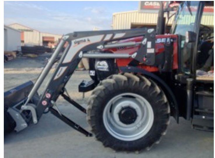
6). Engage the Hand Brake and Switch the Engine Off. Release the Hydraulic pressure from the Valve.
