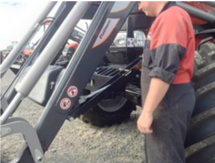
15). Raise the Loader to clear the Support Legs from the ground and Stow the Support Legs away.
