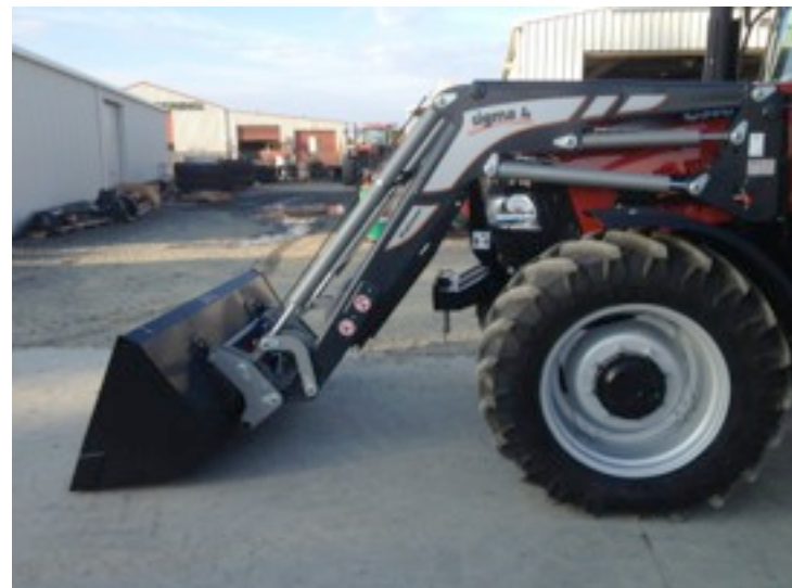
16). The Loader is now Safely Attached and ready for use.
