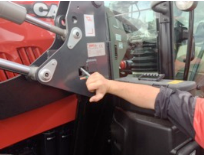
13). Check the Safety Lock Pin has dropped into the Green Position.
