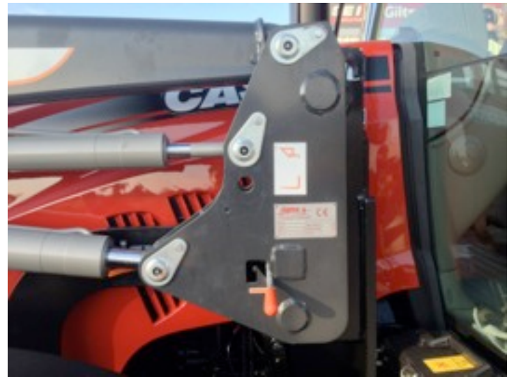
14). Ensure the Safety Lock Pin is Locked in the Green Position.
