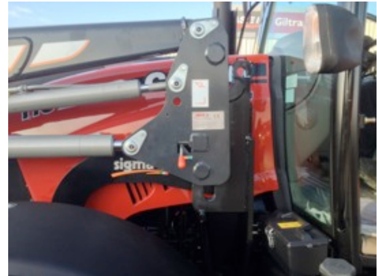
8). The Loader is now completely detached from Frame and the Tractor is ready to be driven away.
