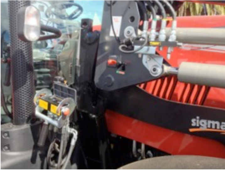
9). Position Tractor in the Centre of the Loader.
