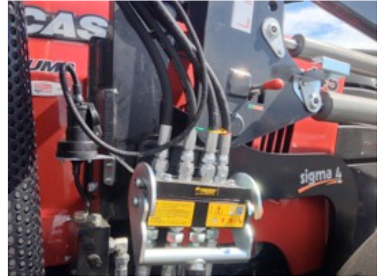
10). Connect the Hydraulic Quick Release Valve and Third Service Plug.
