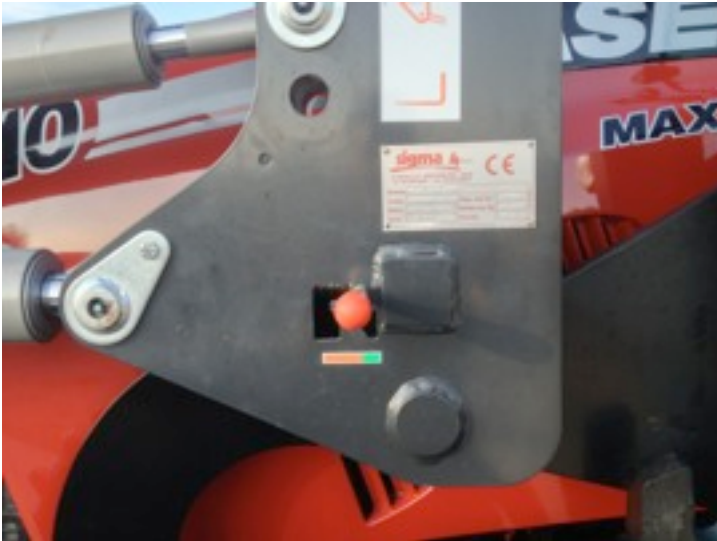
11). Place the Safety Lock Pin in the Central Position.
