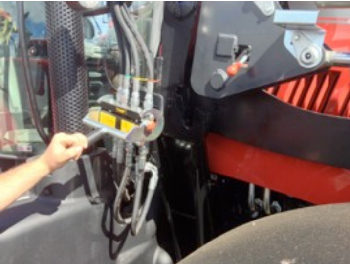
7). Disconnect the Hydraulic Quick Release Valve and Third Service Plug.
