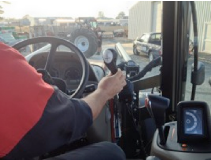
5). Release the Hand Brake. Crowd the Joystick back until the Loader detaches from the Tractor.
